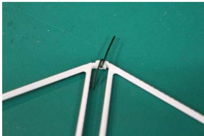
**Step 4.** Glue the tied wings with a piece of light fabric or thin film. Be careful not to use super glue too much, otherwise the 2 wing components will stick together. The thinner the better for the super glue.
