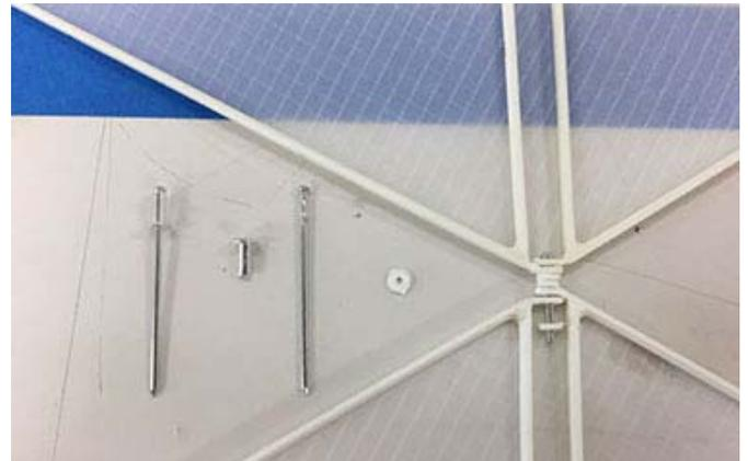
**Step 7.** Connect right cells' top and bottom with the wing ends of the centre cells. Beware that right ends of wings are slightly lowered and left ends are raised to be assembled in correct positions.
