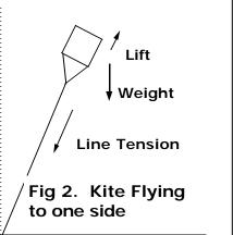
so there is now a force tending to move the kite out of the plane of the lift and the line tension – a small "side force due to gravity". Fig. 3 shows a view looking down on the kite.
