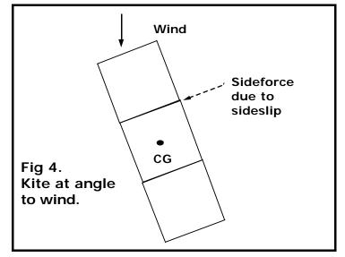
other side. The kite will then move in progressively larger swoops from side to side. If the side force due to sideslip is much too far forward the kite will probably spin on the spot, like an Indian fighter kite on a slackish line.
