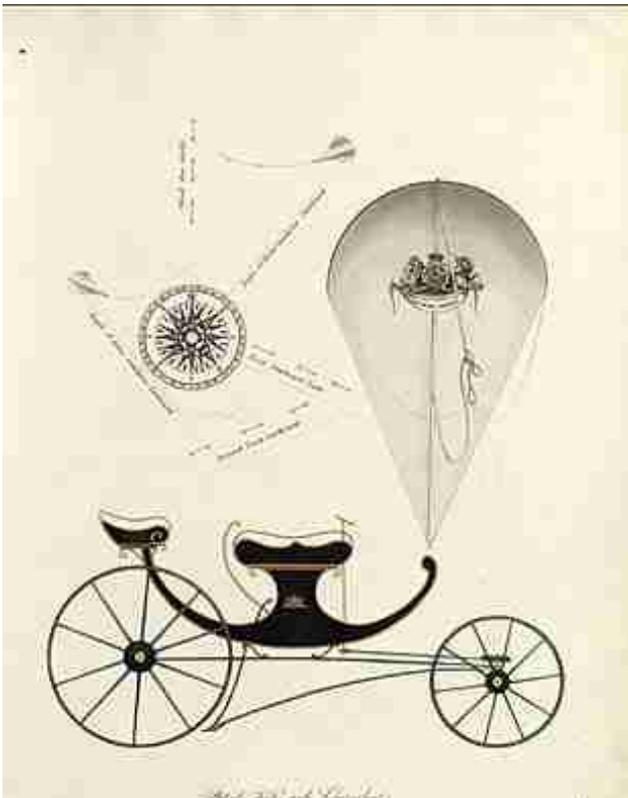
The kite was covered with pink or green glazed calico or linen. It had three wooden parts: the bender (the arched top); the straighter (the spine) in two or three sections the wood about 1" square: the stretcher (spar) which went between the spine and the cover.
