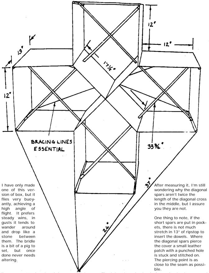
All spars are ¼" dowel and the cover ripstop. The joints I made simply from plastic pipe cut and bent. They don't slip out or anything, not protrude through the cover. It could conceivably be improved by adding another 13" dowel in a sleeve or pockets in the very centre of the cross to keep the cover really taunt. If made bigger twin braces would probably be necessary and the bracing lines on the back which control distortion might be dispensed with.
